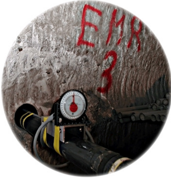
Figure 6.13: Probe setup to determine the rotational characteristics at test site Asse II, borehole EMR3.
