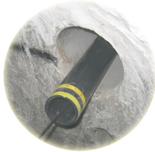
Figure 6.11: Off-center measurement in borehole EMR5 at test site Asse II.
